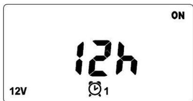
Press "menu" button again, window switch to Timer2 setup interface. Press "enter" button once, you can adjust the "Hour" (1-12hours) via "Page up/Page down" buttons, and then confirm it by pressing "enter". Timer2 hours stands for the time the load will be OFF after Timer1 hours have finished.
