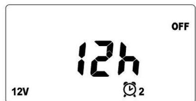
NOTE: When the Timer2 hours are finished, the load will turn ON again until dawn. (See Diagram below)
