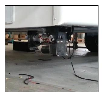
This picture shows the rear jacks have been moved forward to give more ground clearance at the back of the chassis. Note the smooth aerodynamics of the under body.
