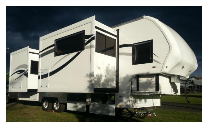
I have tried everything to get the weight down in the 27FLB. Unfortunately without reducing much requested features, it is not possible. The set weight for this model will be 3600kg empty, and 4495 kg loaded. This will give a cargo capacity of 895kg.
